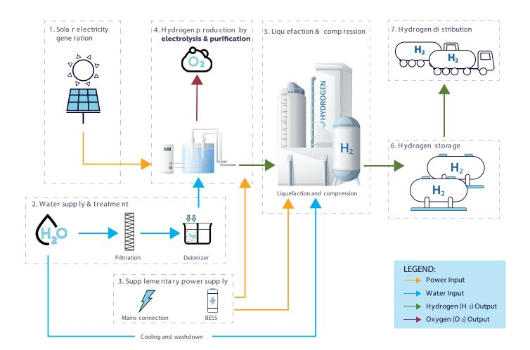
Solar electricity generation: Solar panels would produce up to 250 MW of electricity for the purposes of green hydrogen production
